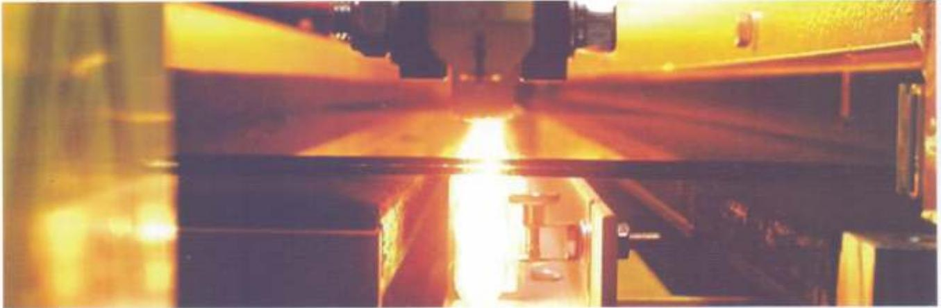
Figure 9 : Infrared Heat for Glass Processing
