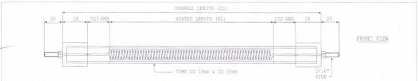
Figure 14 : MWIR Quartz Heater of Size - OD19mm & ID 15mm
