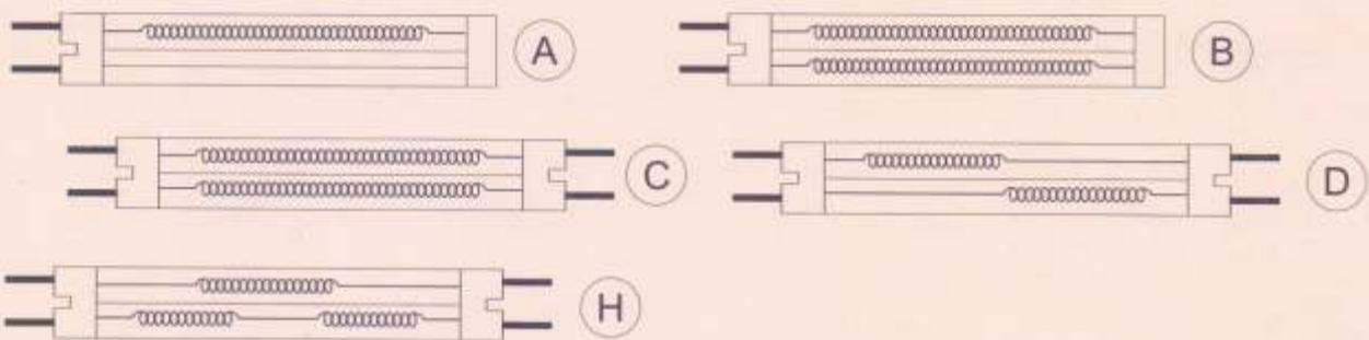
Figure 18 : Type of Twin Tube Medium Wave IR Emitters
