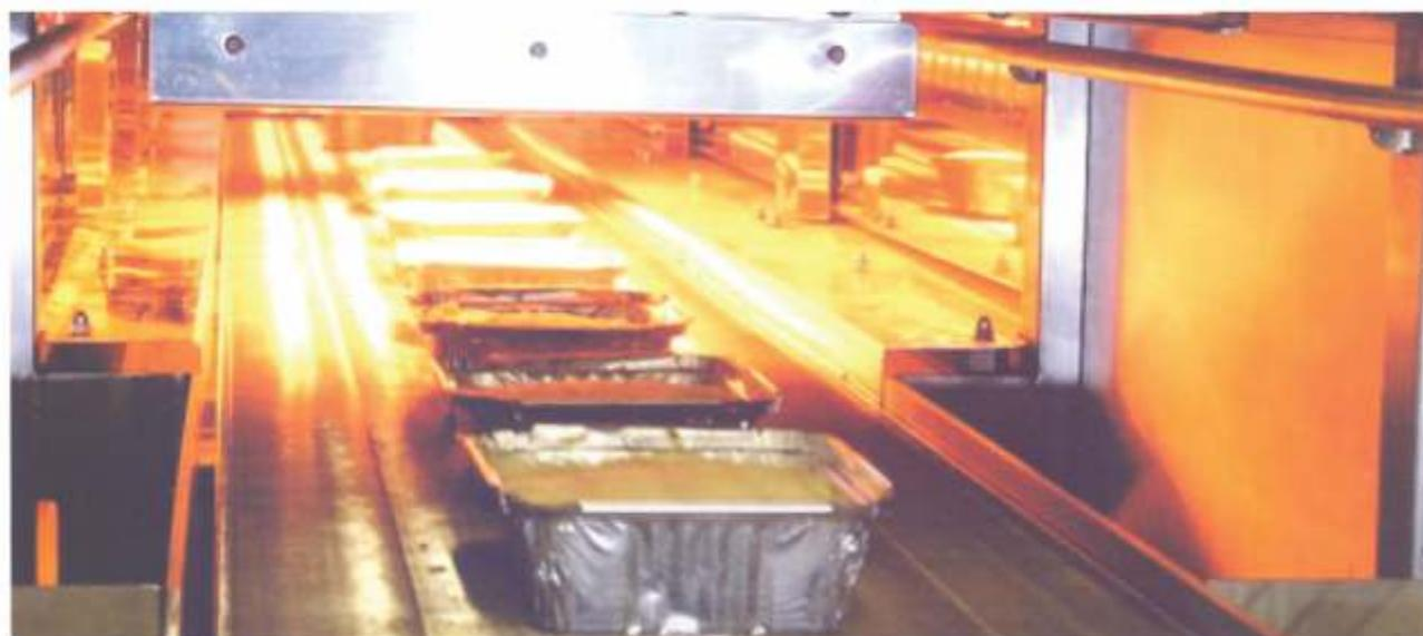
Figure 8 : IR Conveyors
